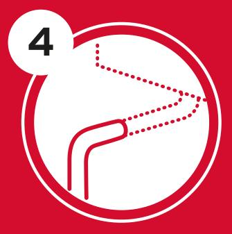
The condensate drainage pipe is a plastic pipe, typically grey or white, connected to the bottom of your boiler. It runs through the wall and outside the property for part of its length.
