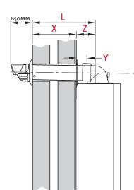
L = Flue length, measured from outside wall face to centre line of flue outlet.
