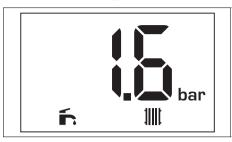
The filling pressure in the heating installation and the operating mode are shown in the display's basic display.
