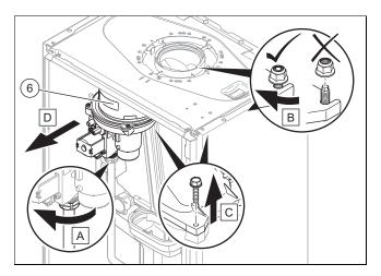
9. Remove the gas-air mixture unit (6).
