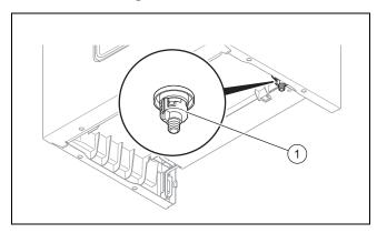
Connect a hose to the drain cock (1) and guide the free end of the hose to a suitable drainage point.
