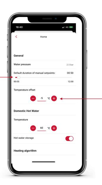
If you observe a gap between the real room temperature and the one measured by vSMART, you can add an offset here
