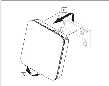
1. Remove the control from the unit mounting bracket as shown in the figure.
