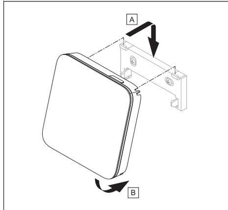
7. Clip the control into the unit mounting bracket as shown in the figure, making sure that it clicks into place.
