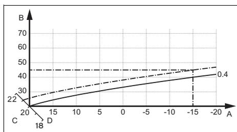
A Outdoor temperature °C      C Target room temperature °C
