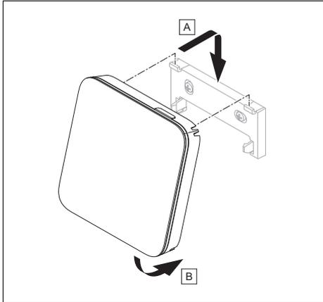
15. Fit the control to the unit mounting bracket as shown in the figure, making sure that it clicks into place.
