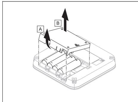
3. Open the control's battery compartment as shown in the figure.
