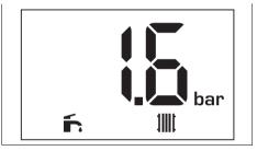
The filling pressure in the heating installation and the operating mode are shown in the display's basic display.
