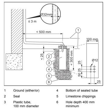
Least preferred option, must not terminate in rain water drain
