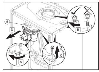
9. Remove the gas-air mixture unit (6).
