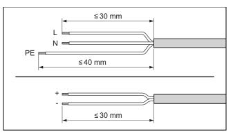
6. Strip the flexible cables as shown in the figure. In doing so, ensure that the insulation on the individual conductors is not damaged.
