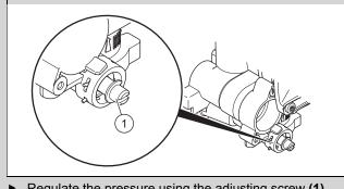
Regulate the pressure using the adjusting screw (1) ►
