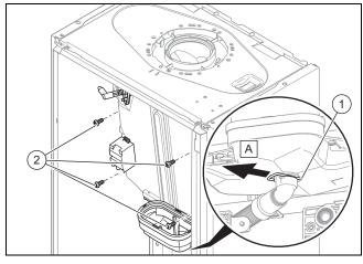
Remove the clip underneath the condensate tray (1).
