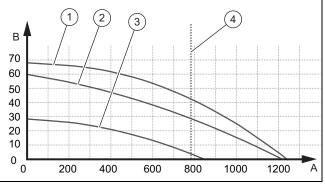
1 Maximum speed (bypass closed) 2 Maximum speed (factory setting for the by-
