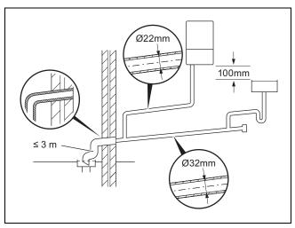
Open end of pipe direct into gulley below ground level but above water level
