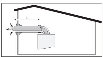
The openings in an attachment for separate lines must lead to a 50 cm-sided square.
