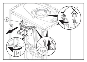
8. Remove the gas-air mixture unit (6).
