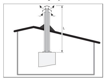
The openings in an attachment for separate lines must lead to a 50 cm-sided square.
