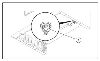
Connect a hose to the drain cock (1) and guide the free end of the hose to a suitable outflow location.
