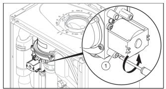
Use a screwdriver to undo the sealing screw on the measuring nipple (1) of the gas valve.
